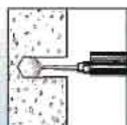
(3) Insert resin outward from the bottom.
