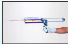
5. Screw mixing nozzle onto cartridge and dispense 2-3 trigger pulls of adhesive to waste until color is red with no streaks.
